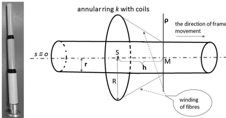
**Fig. 5** Example of a straight-line frame with three parts with different radii of their circle cross-sections on the left. The mathematical model of annular ring  $k$  of the winding head, straight-line frame and winding plane  $\rho$  is shown on the right.
