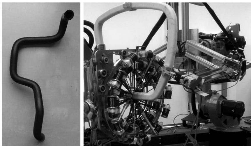
**Fig. 3** Example of a 3D multi-shaped non-bearing hollow frame with circular cross-section (on the left). Closed non-bearing frame prepared to winding process. Frame is connected to robot working arm and goes through winding head (on the right).
