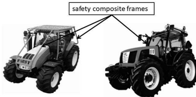
**Fig. 2** Safety composite frames for the tractor cab.
