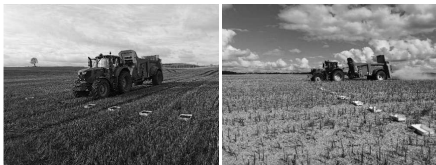
Fig. 2 Arrangement of boxes to determine the evenness of organic fertilizers
