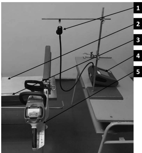
Fig. 1 Layout of experimental setup: 1- sampler, 2 - specimen, 3 - sawhorse, 4 - monitor, 5 - chainsaw
