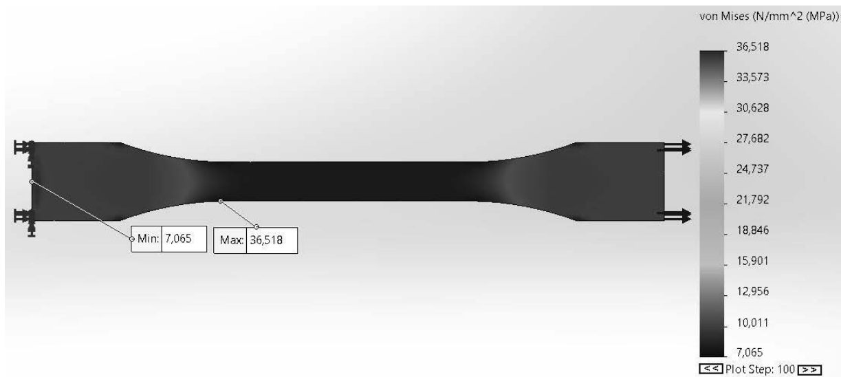
Fig. 3 Result of the simulation with load force 1400 N
